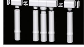
This drawing illustrates some of the customizable filter connection options the ERO 385 has to offer. Additional filter(s) may be added on to either side
